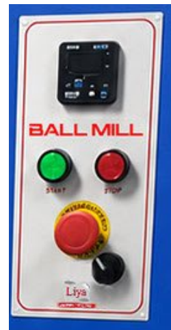
Operating controls and emergency stop
