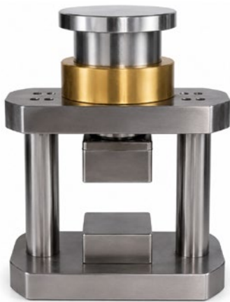
Compression test jig and loading faces
