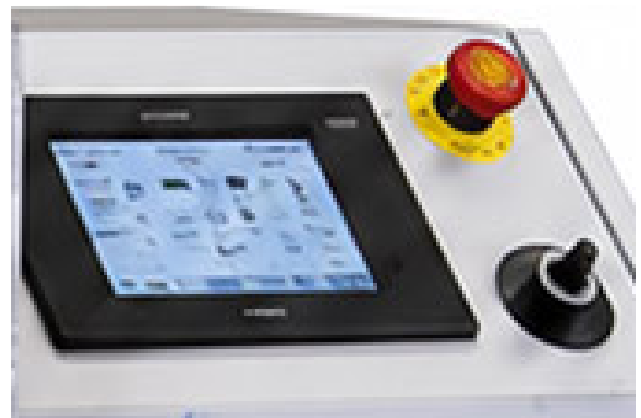
Touchscreen controller and emergency stop
